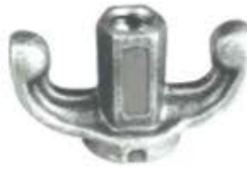
FORGED WING NUT Material : EN-8 Weight : 0.350 Kg Working Load : 90 Kn
